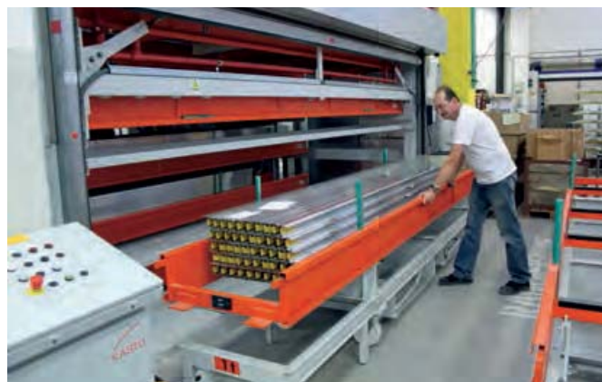
A cassette is moved out of the outfeed station, in which the OGC has placed the cassette onto a moving transport fixture. One of the two RFID transponder chips is visible at the front side of the cassette.
