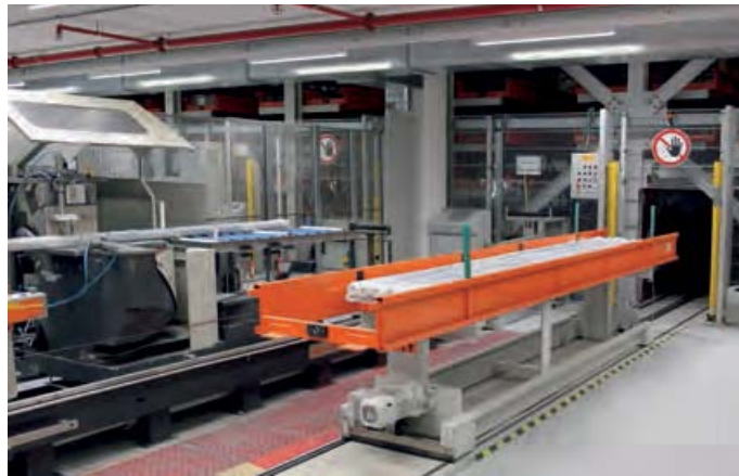
The removal station at the CNC-profile processing centre for individual removal of one or several profiles directly at the machine
