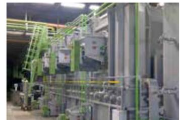
Category: **INDIRECT HEATING GAS-FIRED FURNACE for ALUMINUM BILLETS**
