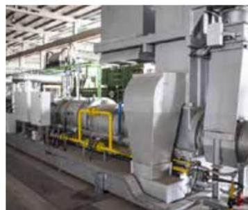
Category: **GAS-FIRED HEATERS for ALUMINUM LOGS with HOT SHEAR or HOT SAW**
