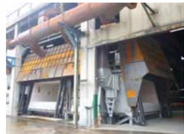
The furnace is designed so that skimming operations are performed through a small side door of the cold chamber, allowing fast skimming and reduced heat loss.
