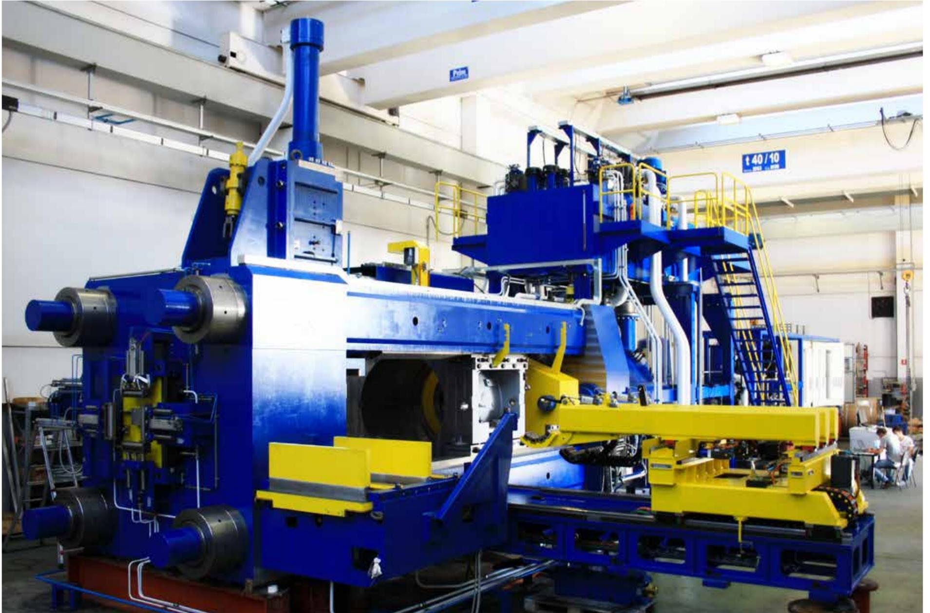
Pennex has successfully commissioned a 55 MN front loading extrusion press supplied by Prezezzi Extrusion at its works in Leetonia. This press is a front loading, short stroke one fitted with a container for extruding 12" aluminum billets up to 60" long.
