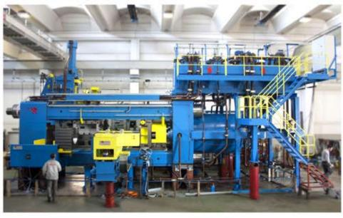
The new PRESEZZI press is 66 MN back loading press that can handle billet up to 60 inches in length.
