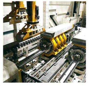
Subsequently another groundbreaking ideas have led to the engineering of a special product for billet heating using the magnetic effect generated by permanent magnet rotation around the metal to be heated.
